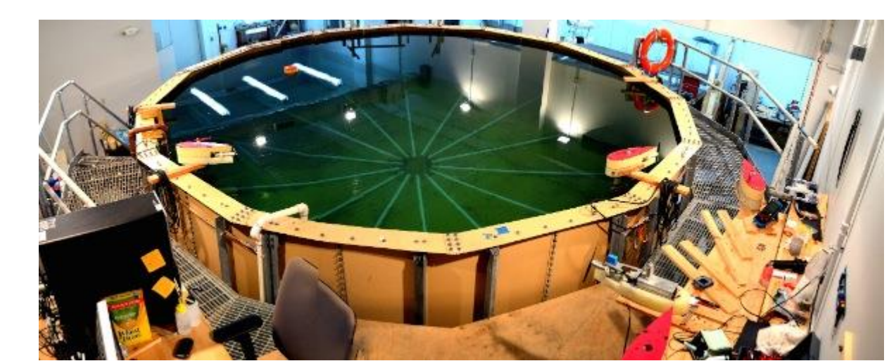
Testbed with tank and underwater vehicles. Credit: Peter Landgren
